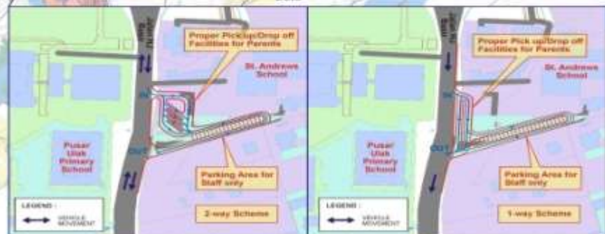
Conceptual Solution - Provision of proper pick up/drop off and parking facilities to solve school peak congestion.
